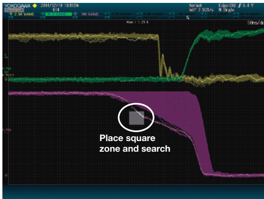
Searching for waveforms that pass through or do not pass through a rectangular zone placed on screen.
