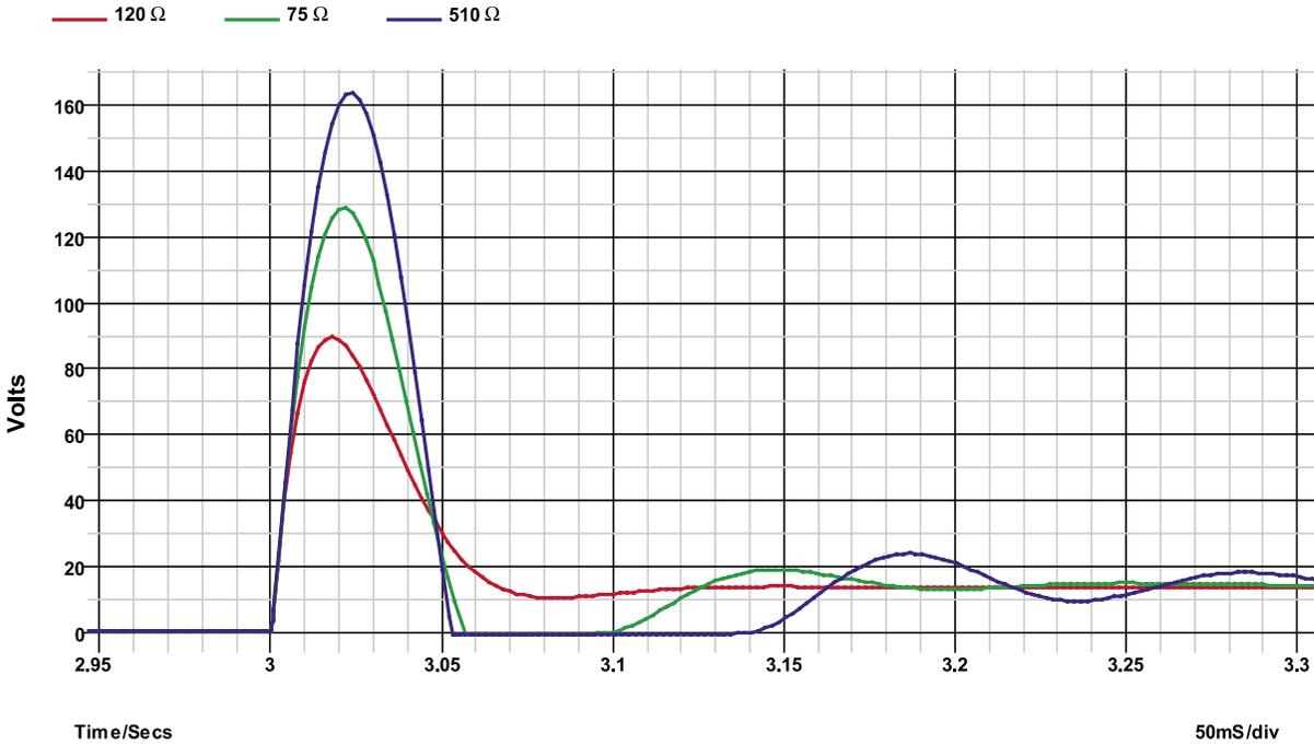
**Figure 4.** Inductor coil current with different values of resistive damping
