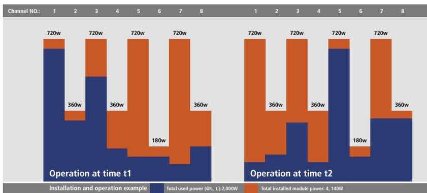
The XMP offers power flexibility, allowing users to draw available power from different channels at different times from the same power system. It is available with 2.4 kW continuous and 2.6 kW intermittent usable power. To ensure the power envelope is not violated, the XMP controller constantly
