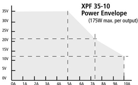
The maximum current at any voltage setting is limited by the power envelope which is set to give 5A at 35V rising to 10A at 12V under all AC supply conditions (both outputs loaded). At lower voltages the power is restricted by the 10 amps current maximum.
