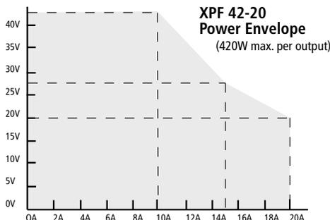
The maximum current at any voltage setting is limited by the power envelope which is set to give 10A at 42V rising to 20A at 20V under all AC supply conditions (both outputs loaded). At lower voltages the power is restricted by the 20 amps current maximum.
