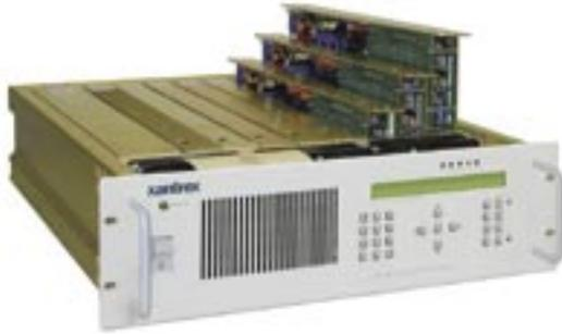
Power modules come in a variety of sizes and power ratings: 1/8 width, ranging from 160 W to 720 W; 2/8 width, ranging from 640 W to 1.6 W; and 3/8 width high power modules ranging from 2.8 kW to 3.2 kW, limited by the XMP mainframe power envelope.
