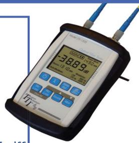
The LTS-1500 is a small, rugged automated fiber optic loss test set that characterizes singlemode and multi mode fiber links at wavelengths of 850,1300, 1310, 1490 and 1550 nm, The power meter uses a sensitive InGaAs detector that is calibrated at six wavelengths with an 80+ dB dynamic range. The Light source is a single port system with up to three wavelengths.
