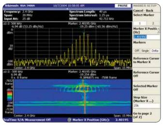
High-resolution spectrogram reveals transient signal behavior that translates to rapid problem solving. Here, 500 kHz sidebands are revealed as part of the transient behavior of a hopping signal as it switches frequencies.
