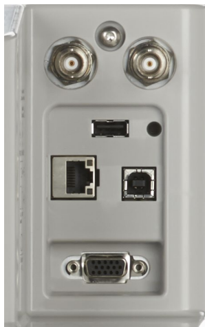
Figure 52. Connectivity section on the back panel.
