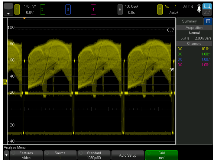
Figure 45. Triggering on a 1080p/60 signal.
