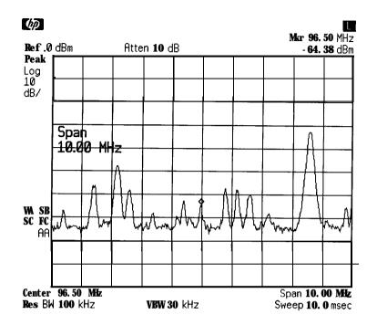
**6. Press Amplitude, Attenuation Auto Man.** Press the step-up key (<sup>†</sup>) twice to select 20 **dB** attenuation. Increasing the attenuation moves the noise floor closer to the signal.
