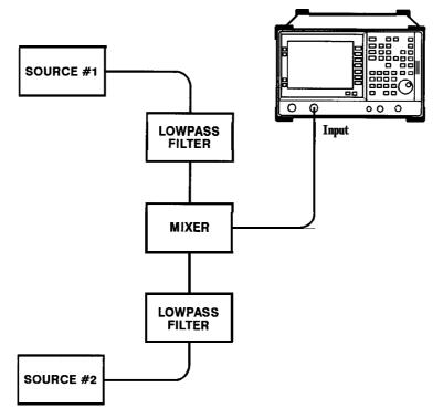
Figure 2-22 Third-Order Intermodulation Equipment Setup
