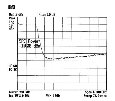
Figure 3-2 Tracking Generator Output Power Activated
