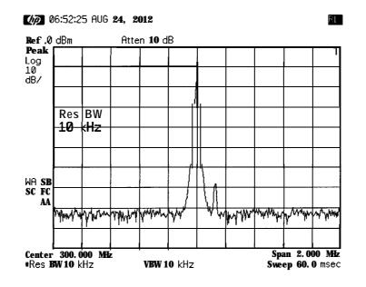
If a 30 kHz filter is used, the 60 dB bandwidth could be as wide as 450 kHz. Since the half-bandwidth (225 kHz) is wider than the frequency separation, the signals most likely will not be resolved. See Figure 2-8. (In this example, we used the 60 dB bandwidth value. To determine resolution capability for intermediate values of amplitude level differences, assume the filter skirts between the 3 dB and 60 dB points are approximately straight.)
