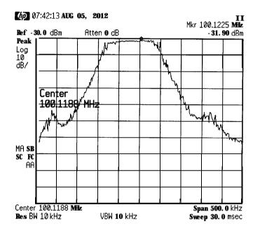
Annotation on the left side of the screen indicates the trace mode. For example, MA SB SC indicates trace A is in maximum-hold mode, trace B and trace C are in store- blank mode. See "Screen Annotation" in Chapter 1.
