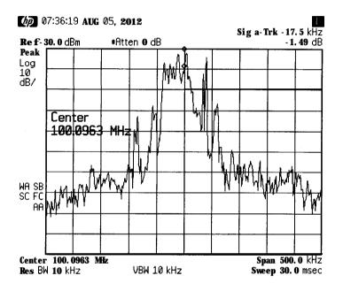
The spectrum analyzer can measure the short- and long-term stability of a source. The maximum amplitude level and the frequency drift of an input signal trace can be displayed and held by using the maximum-hold function. You can also use the maximum hold function if you want to determine how much of the frequency spectrum an FM signal occupies.
