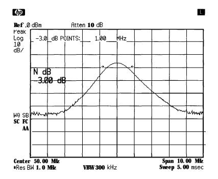
**Example:** Measure the 3 **dB** bandwidth of the spectrum analyzer's 1 MHz resolution bandwidth filter using the internal 50 MHz signal.
