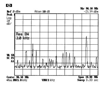
A # mark appears next to the **Res BW** annotation at the lower left corner of the screen, indicating that the resolution bandwidth is uncoupled.
