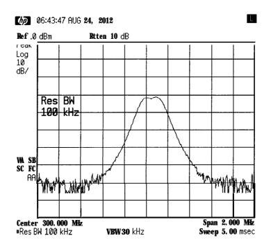
As the resolution bandwidth is decreased, resolution of the individual signals is improved and the sweep time is increased. For fastest measurement times, use the widest possible resolution bandwidth. Under preset conditions, the resolution bandwidth is "coupled" (or linked) to the span.
