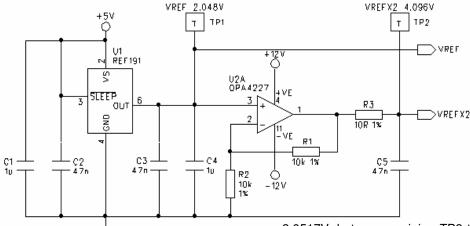
Using a DVM, the voltage at TP1 measures correctly at 2.052V (which is within tolerance). but at TP2 something very strange is happening. The test point voltage measures about 4.1V but the DVM reading is unstable - the last couple of digits are changing all the time. What's going on?
