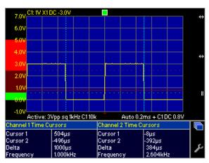
On the third waveform (on the right), an invalid signal is shown. Here the high logic level is only about 2V, which is below the valid high level threshold as can be clearly seen on the display. The high level is in "no man's land" and may well be due to an overloaded output, bus contention in a tristate circuit, or a faulty IC output.
