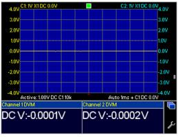
Let's explain. The CircuitMaster uses *Active* mode to impose an active load on the probe, using a programmable voltage source in conjunction with a selectable series resistance. With an open circuit, the input voltage follows the active load voltage (1V nominal, actually 0.9842V measured by the DVM), but with a short circuit the input is still 0V as in the right hand picture.
