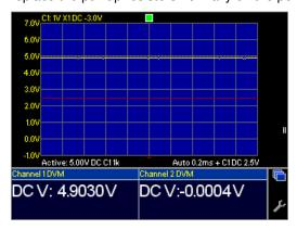
■ Here is the result for the driver with a faulty open circuit output. The output is pulled to 5V by the active pull-up in the CircuitMaster. and the results is a horizontal line at 5V and a 5V (approx) DVM reading.
