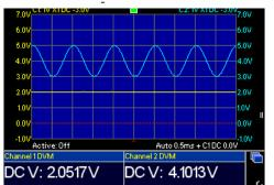
as 2.0517V, but on examining TP2 the problem becomes clear – the voltage is oscillating (upper trace) because the op amp U2 is unstable. The DVM measures the  ${\bf average}$  voltage, which  ${\bf looks}$  correct, but the oscilloscope shows the oscillating signal clearly
