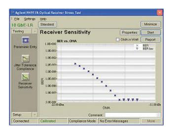
Figure 32: Optical receiver stress testing with N4917A allows calibrated stressed receiver sensitivity tests
