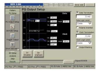
Figure 13: Pattern generator setup screen with graphical display of signal levels.
