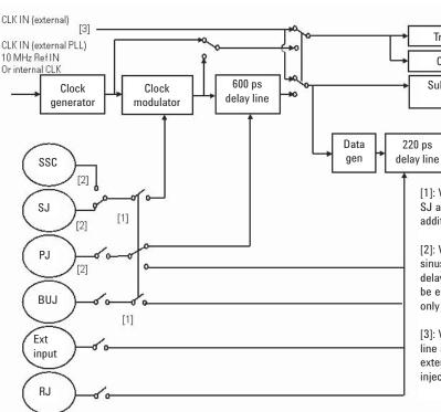
[1]: When 600 ps delay line is used for PJ, additional SSC, SJ and BUJ is not available. The 220ps delay can be used in addition, see above for maximum available total jitter.
