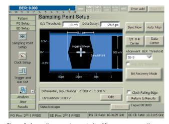
Figure 9: Auto alignment (center) simplifies correct sampling even for stressed eyes.
