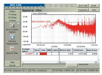
Figure 5: Spectral jitter decomposition for debugging jitter sources in a design.
