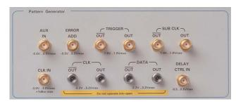
Figure 11: Generator connectors on front panel
