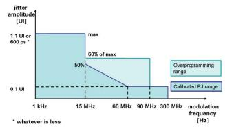
Figure 22: Periodic jitter maximum for datarates  $\leq$  3.375 Gb/s using the 600 ps delay line.
