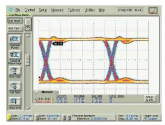
Figure 12: Clean output signal. 10 Gb/s, LVDS levels.
