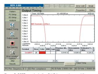
Figure 7: BERT scan including RJ/DJ separation, total jitter.
