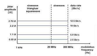
Figure 21: Periodic jitter maximum for all data rates using the 220 ps delay line.
