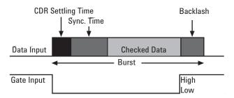
Figure 20: Burst mode allows recirculation loop testing.
