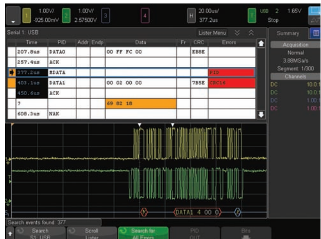
Figure 21. USB 2.0 trigger, decode and "lister" display.
