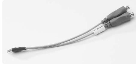
**12 GHz Hi-BW solder-in differential probe head** provides maximum bandwidth and minimizes capacitive loading to  $\leq 210$  fF. Variable spacing from 0.2 to 3.3 mm (8 to 130 mills).
