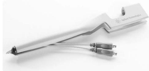
**12 GHz Hi-BW differential browser** provides maximum bandwidth for hand-held or probe holder use. Variable spacing from 0.2 to 3.3 mm (8 to 130 mills).
