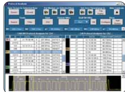
► CAN and LIN Timing and Protocol Decode.
