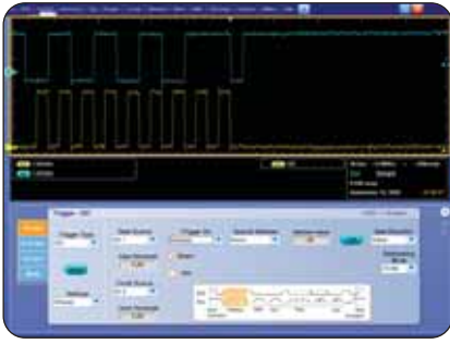
► Easily trigger on a specific I 2 C address.
