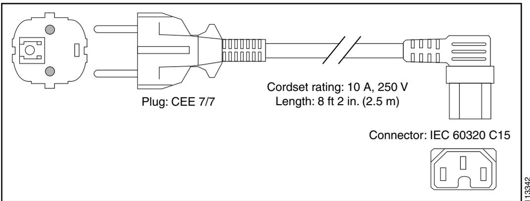
**Figure A-22 CAB-AC10A-90L-IT= (Italy)**
