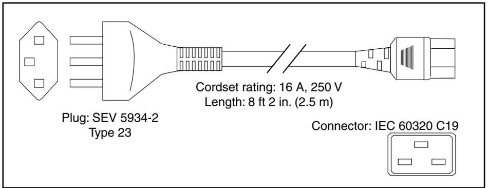
**Figure A-46 CAB-AC-16A-AUS= (Australia and New Zealand)**
