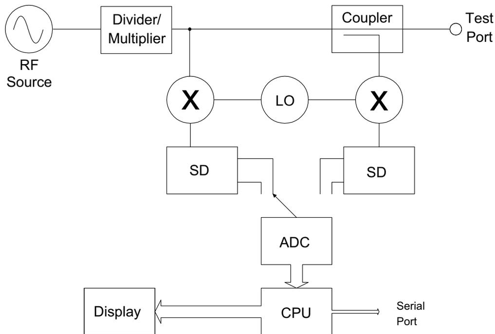
**Figure 2.** Site Master Block Diagram
