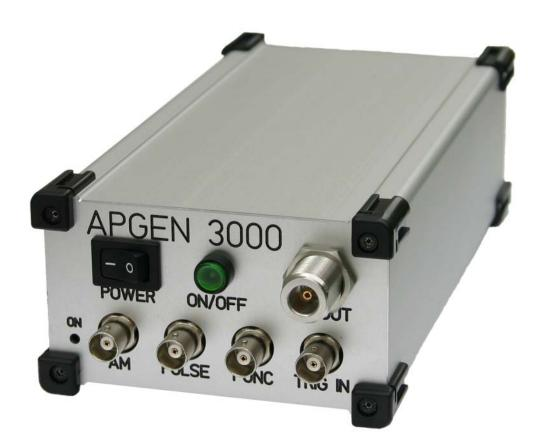
The APGEN3000 is a fast-switching RF Signal Generator with dedicated modulation and trigger capabilities. The APGEN3000 covers a frequency range from 9 kHz to 3.0 GHz and is ideally suited for a wide range of application, where good signal quality, fast switching, and accurate and wide output power range is required.
