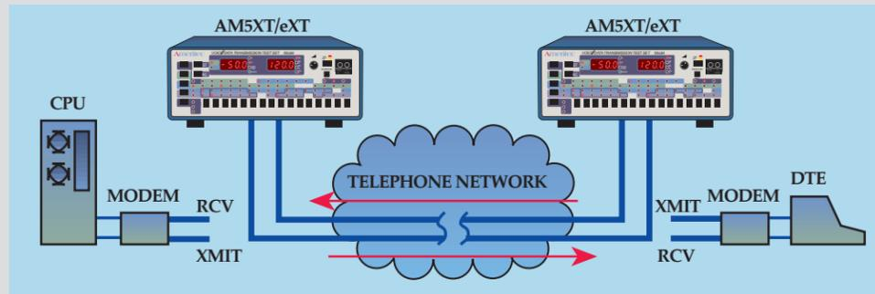
Use a single unit with an Ameritec AM3 Series 4 Wire Responder for centralized loopback testing.
