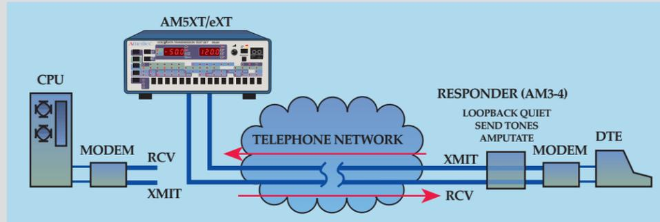
Use the AM5XT/eXT built-in dial capability on dial-up networks to access a distant Ameritec AM3 Series 2 Wire Responder or a second AM5XT/eXT for centralized 2 wire testing.
