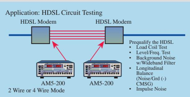
Use two sets for a complete end-to-end test of 4 wire data lines.
