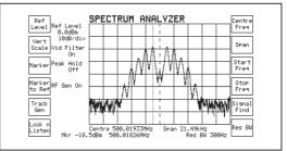
The spectrum analyzer provides spans from 100 Hz per division to 100 MHz per division and also has a fully adjustable reference level. Speed is comparable with analog analyzers, allowing real time adjustments over the displayed dynamic range. With the tracking generator provided as standard, duplexers and filters can be aligned quickly and easily. An offset facility provides testing of equipment with fre-
