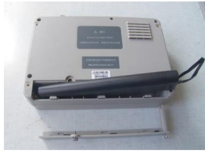
Fig.1.1 Battery compartment door
