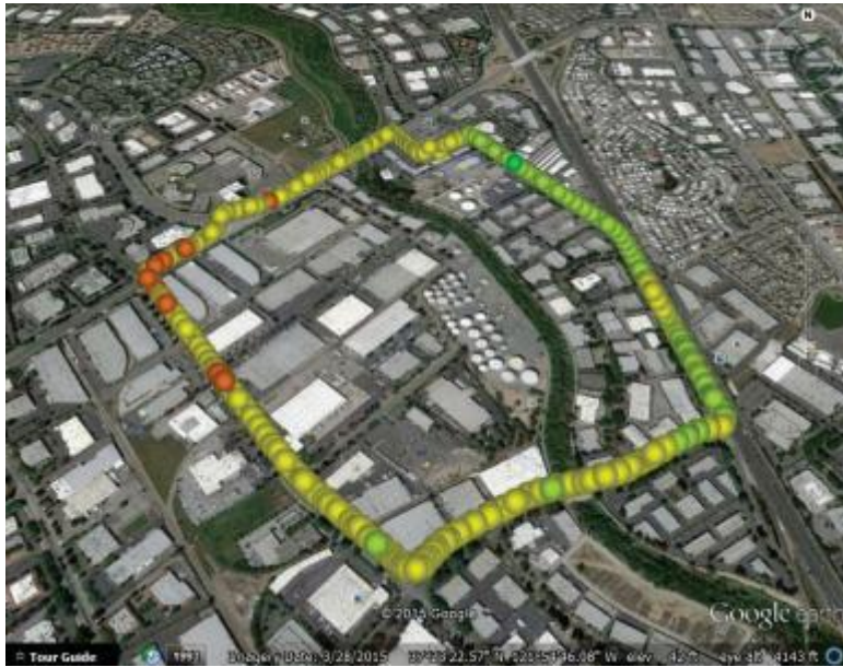
Fig.32.6 Outdoor coverage survey in .KML format, displayed in Google Earth
