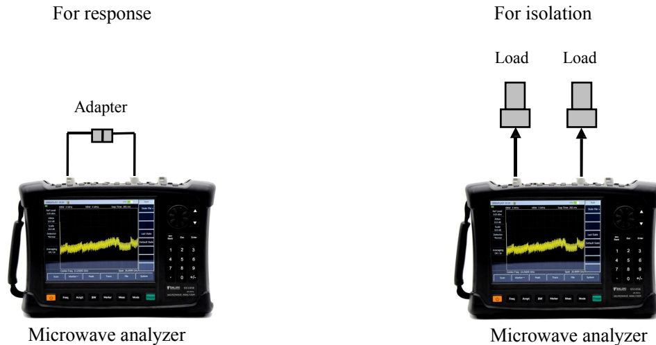
Figure 4-5 Standard piece connection for transmission measurement response and isolation error correction
