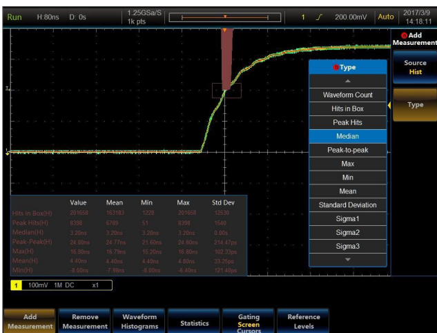
Horizontal histogram: to observe jitter and jitter distribution of signals.
