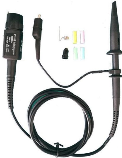
P9350A passive voltage probe (H14)
