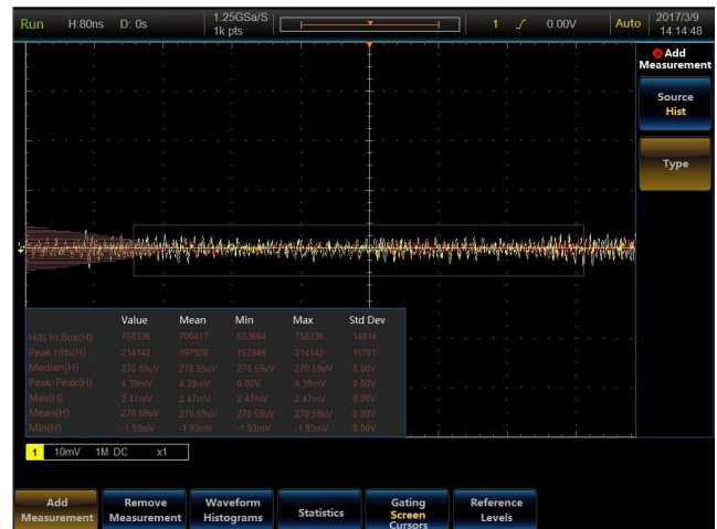
Vertical histogram: to observe noise and noise distribution of signals.
