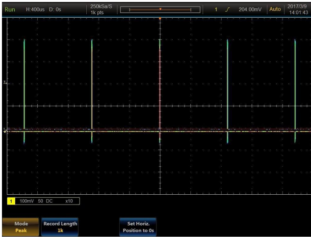
The smallest pulse capture width is 200ps.
