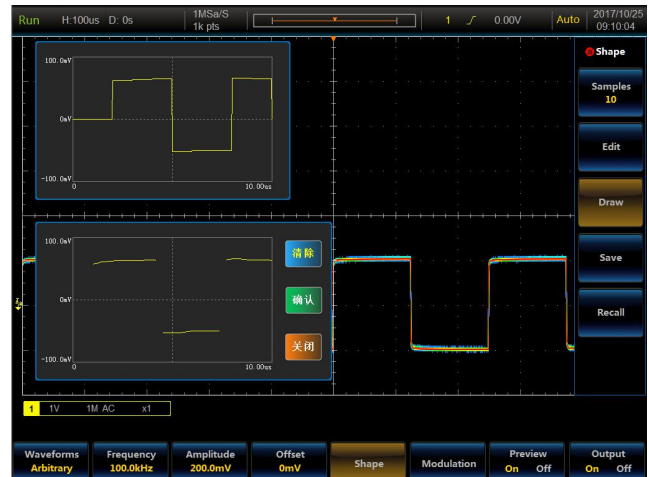
The capacitive screen can draw arbitrary waveform output quickly.
