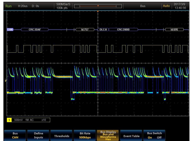
Serial protocol trigger: I2C, SPI, RS232, CAN, LIN, FlexRay, Audio, USB.
