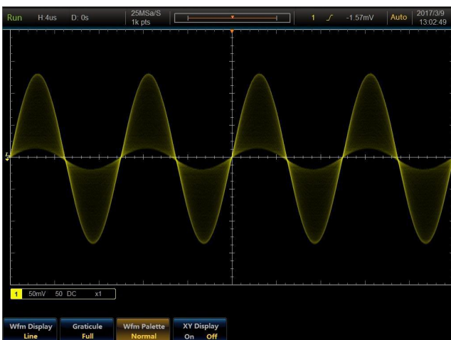
Normal: indicates event probability by default channel color and gray scale. Bright color indicates events of high occurrence probability.
