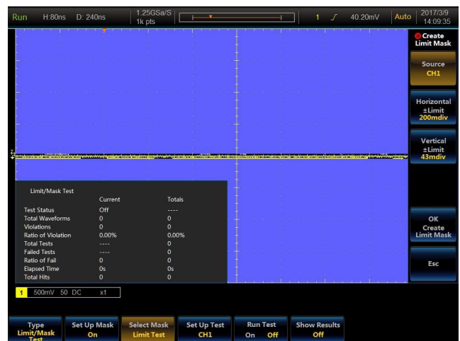
Limit and mask test: standard and custom mask, pass/fail test, result display.
