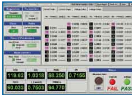
IEC 61000-3-2 Current Harmonic Test
